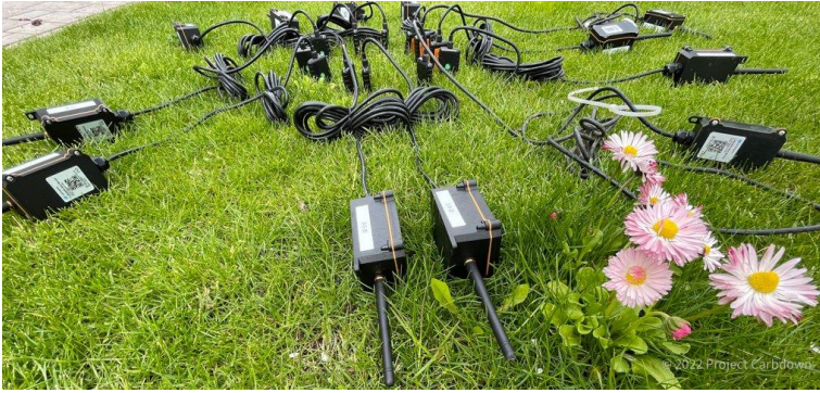
Underground, sensors in which the radio module and the probe are connected with a robust cable are suitable (Photo: Project Carbdawn).
